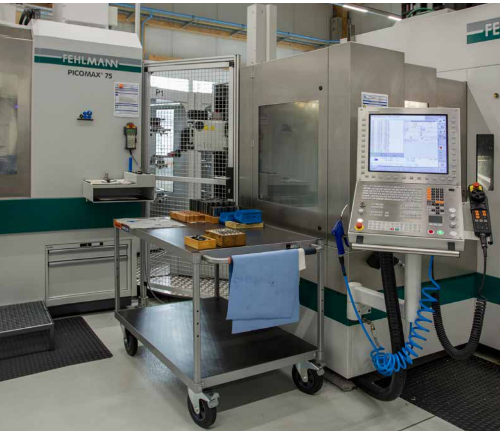
Standard setup: two machines with a pallet system enable unattended shifts at night and on the weekend.
