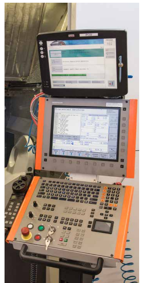
The iTNC 530 and the shop floor management system are directly connected for automatic recording of machine data.
