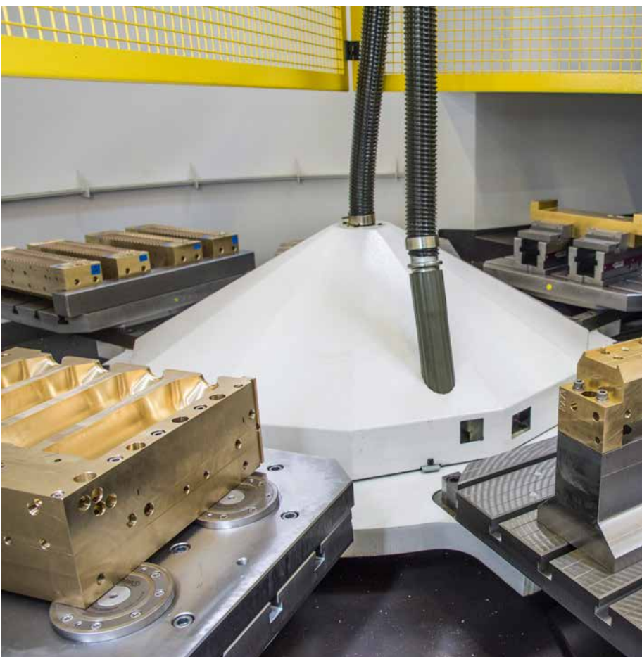
A compact, easily accessible pallet changer from GF Machining Solutions.
