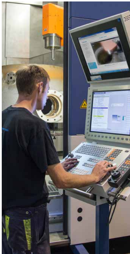
Ideal for high-precision, full-surface machining: The TNC 640 in the Grimsel Hydro maintenance workshop.
