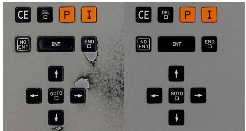
It’s the customer’s choice: Functional repair (left) or premium repair (right) are both technically optimal.
