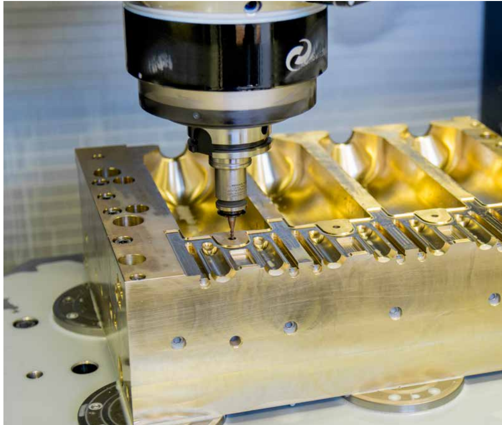
Machining a bottle form with spherical end mills takes many hours, but is process-safe thanks to the iTNC 530.
