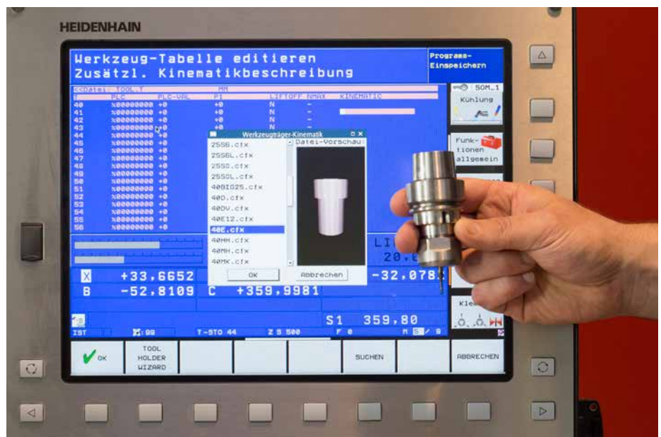
A broad and comprehensive solution—DCM collision monitoring, in addition to considering fixed machine components, also monitors tools and tool carriers...
